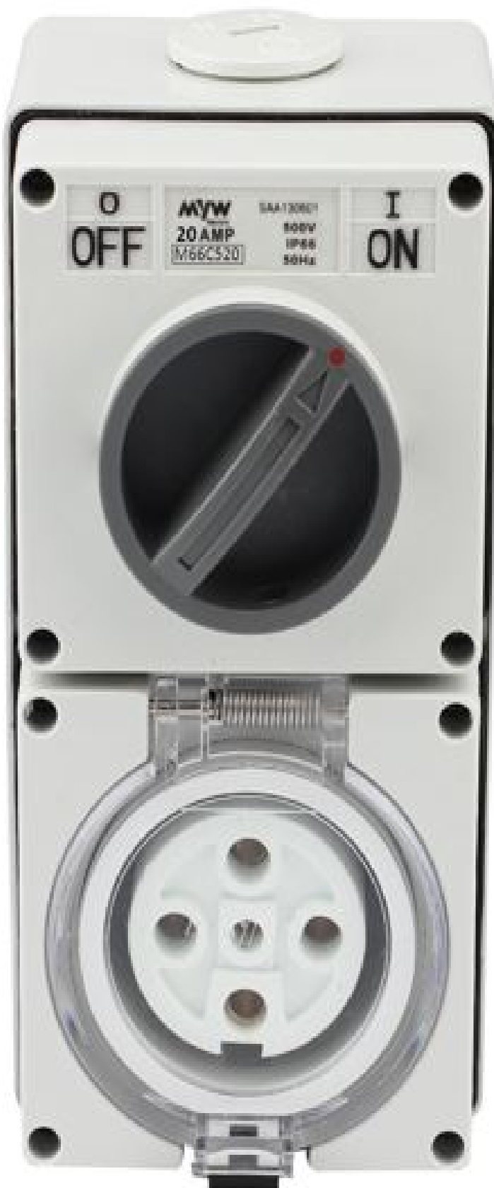
SWITCHED SOCKET OUTLET COBINATION 20 AMP 500V 5 ROUND PIN IP66.
